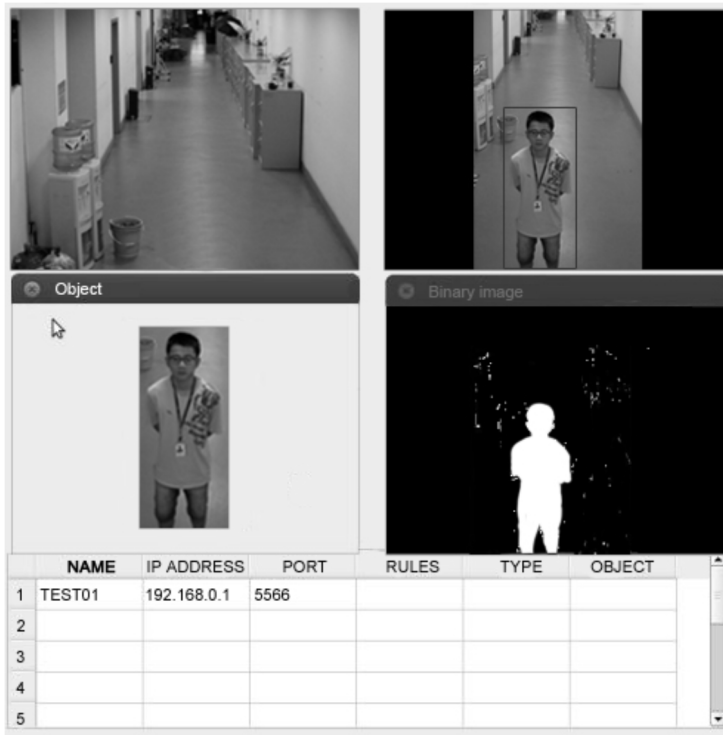
Fig. 3. The monitoring results of the moving objects using intelligent video analysis system
